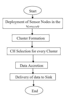
Figure 2: System Model for Clustering in WSN
