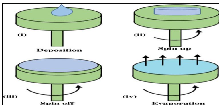
Figure 3. Stages of spin coating on substrate [24]
