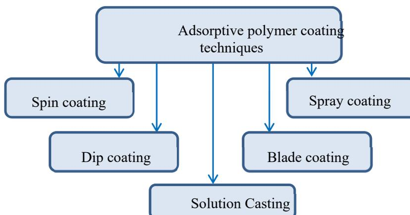
Figure 2. Adsorptive polymer coating techniques [23]
