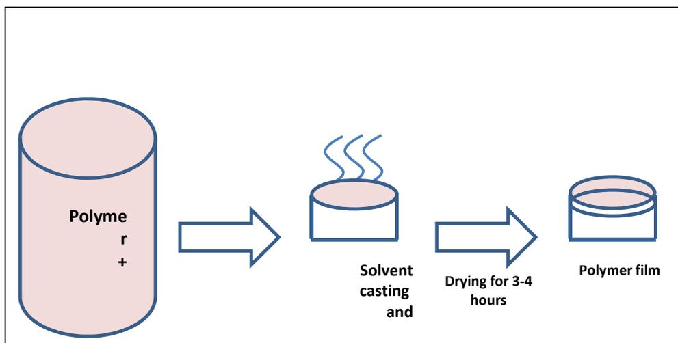
Figure 7. Steps of Solution casting technique [42]
