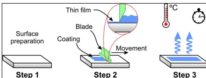
Figure 6. Steps of blade coating technique [37]
