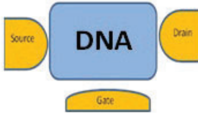
Fig.(1): Schematic diagram of the Single Electron Transistor (SET).
