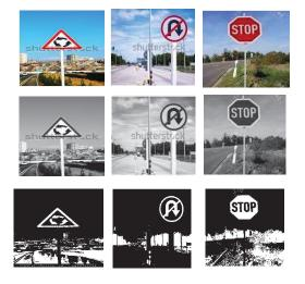
Figure (4): Detection phase of traffic signs
