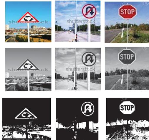
Figure (4): Detection phase of traffic signs
